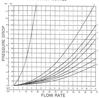
Above curves based on 100 SUS fluid viscosity @ 120° F., .87 specific gravity.
