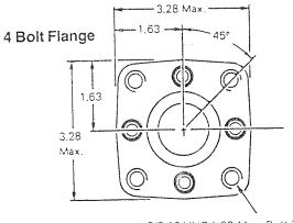
3/8-16 UNC (.60 Max. Bolt Thread Engagement ) Mounting Holes (4) Equally Spaced on 3.25 Dia. Bolt Circle
