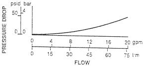
Pressure drops shown are based on 100 SUS fluid viscosity and 0.87 specific gravity.
