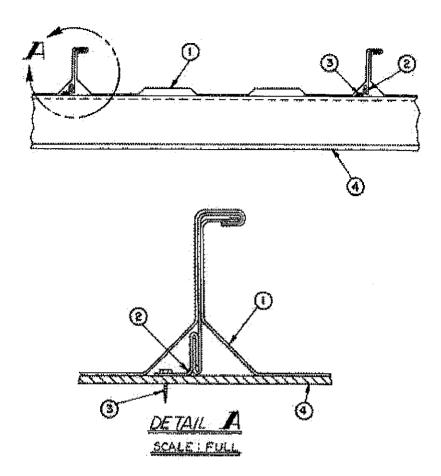
1. **Metal Roof Deck Panels\*** — No. 24 MSG min thick coated steel, 18 in. wide, 2-1/2 in. high at the ribs. Panels continuous over two or more spans without end laps. A line of sealant may be used along panel side joints. Adjacent panels to be seamed together along sides using an electric seaming tool with seams to be fully crimped. Seaming operation to include Roof Deck Fasteners (Item 2 or 2A).
